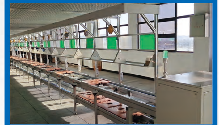
Vertical loop high-speed chain assembly line
