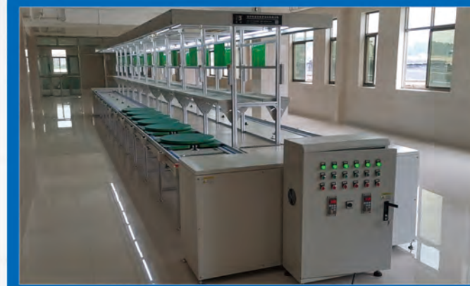
Horizontal loop high-speed chain assembly line
