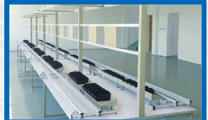
Double-sided non-powered insertion line
