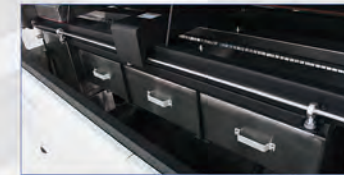
Modular preheating system
