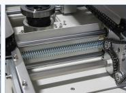
Linkage type width adjustment mechanism
