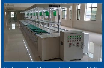
Horizontal loop high-speed chain assembly line
