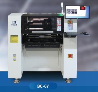
Number of Mounting Heads: 6 Model: BC-6Y Feeder Slots: 66 Positioning Accuracy: 0.02mm Camera: Flying Camera PCB Size: 500×400mm Normal CPH: 12000 Motor/Drive: Servo System Mounting Head Structure: Independent Direct Drive Transmission Main Shaft: Ground Screw + Linear Guide Control Configuration: Industrial Computer + 19" Display Screen
