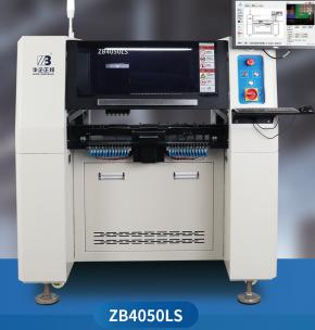
Model: ZB4050LS Number of Mounting Heads: 6 Positioning Accuracy: 0.02mm Feeder Slots: 64 Camera: Fixed Camera PCB Size: 500×400mm Normal CPH: 11000 Motor/Drive: Servo System Mounting Head Structure: Swing Hip Drive Transmission Main Shaft: Ball Screw + Linear Guide Control Configuration: Industrial Computer + 19" Display Screen
