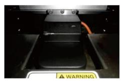
▶平台高度根据PCB板厚设定自动校准,智能快速,结构简单可靠。 The platform height is automatically calibrated according to PCB thickness setting, which is intelligent, fast, simple and reliable in structure.
