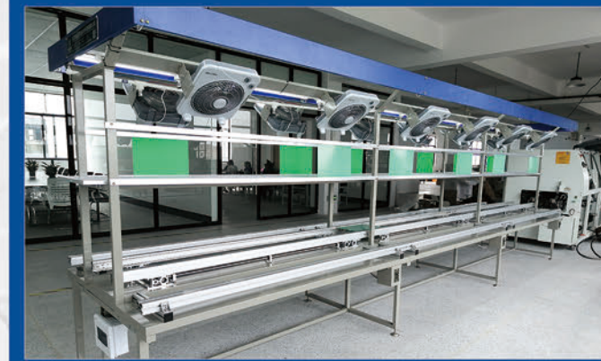
Double-sided automatic insertion line
