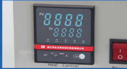
Using PID(Micro-computer) Temperature Control System
